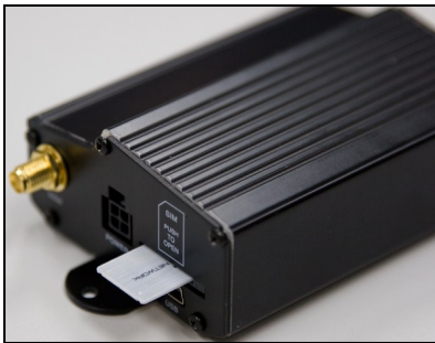
Figure 6. Insert SIM Card into Dialler
